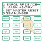
Use the up & down buttons to Select ENROL RF DEVICE Press Enter
