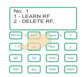
Press button 1 to Learn in an RF Remote control device to the units memory.
