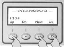
Use the **Up**, **Down** and **Next** button to enter the PIN no: The default is 1;2;3;4. Pin no's can be changed in the Main menu on option [7]
