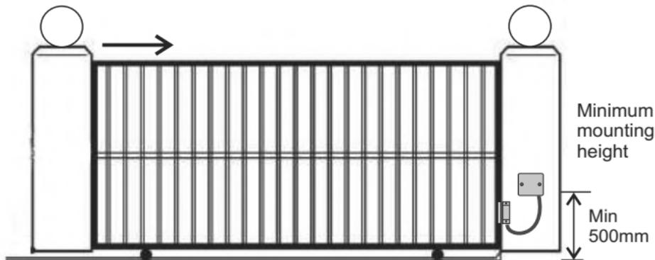
Securely mount & screw the Magnet to the end of the Gate. Align the Wide Gap Reed switch as close to the magnet as possible and securely mount & screw the unit to the wall or post of the gate. Once this is done, position the Gate Alarm transmitter housing slightly above the reed switch onto the wall or post.
